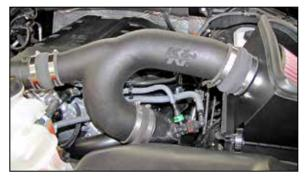
17. Install the K&N® intake tube into the couplers at the turbo inlet tubes and then into the coupler at the filter adapter, adjust the tubes for best fit and then secure with the provided hose clamps.
