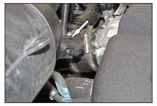
2. Disconnect the inlet air temperature sensor electrical connector and remove the tape around the harness connector.
