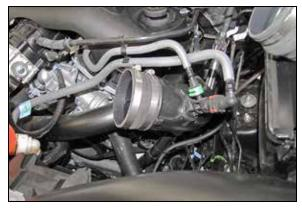
13. Install the provided coupler (08761) onto the driver's side turbo inlet tube and secure with the provided hose clamp.
