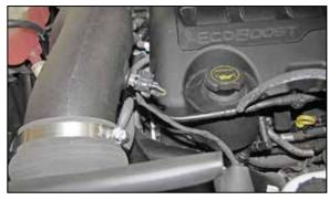
18. Reconnect the inlet air temperature sensor electrical connection using the provided extension harness.
