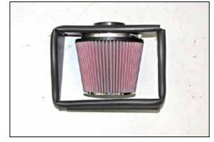
10. Install the K&N® air filter onto the filter adapter and secure with the provided hose clamp.
